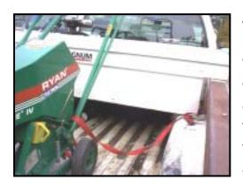
Just as you did when you unloaded the machine from the back of the truck, get a coworker to help you lift the aerator into the back of the truck. Remember to bend your knees as you lift. Once the aerator is positioned in the truck, use four tie-down straps to secure the aerator to the truck ensuring it can't move around during transport.
