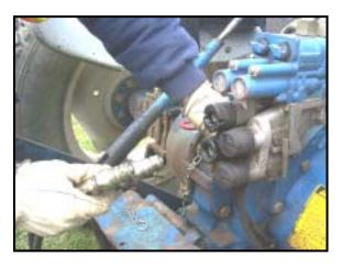
3. The next step is to connect the aerator hydraulics to the tractor.
