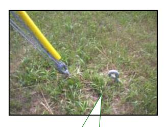
This exposed pin could cause significant damage to a mower or trimmer.
