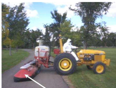
The Windfoil is attached to the Cushman or a tractor.
