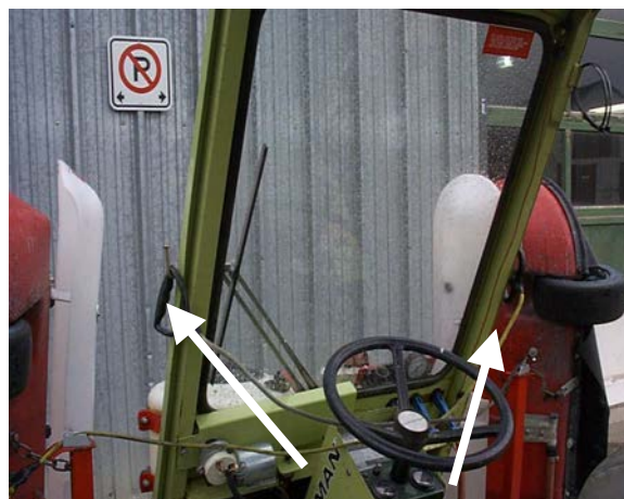
Handles are hooked on the opposite side of the cab.
