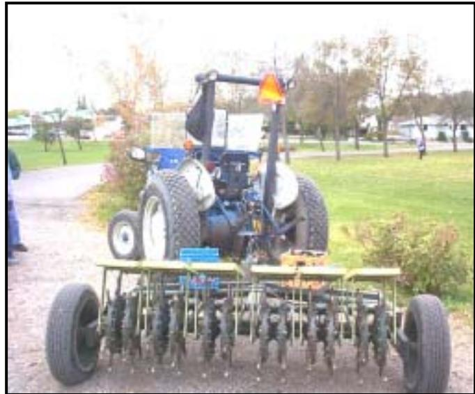
When pulling the aerator on streets, always be conscious that the aerator is wider than the tractor. Keep this in mind when turning corners or moving past another vehicle.
