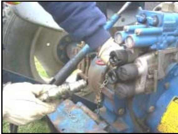
3. The next step is to connect the aerator hydraulics to the tractor.
