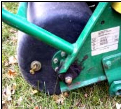
2. Once you've placed the aerator safely on the ground, add water to the drum that's located at the front of the machine. This adds weight to the machine helping the tubes (or tines) to break through the soil easier and deeper.
