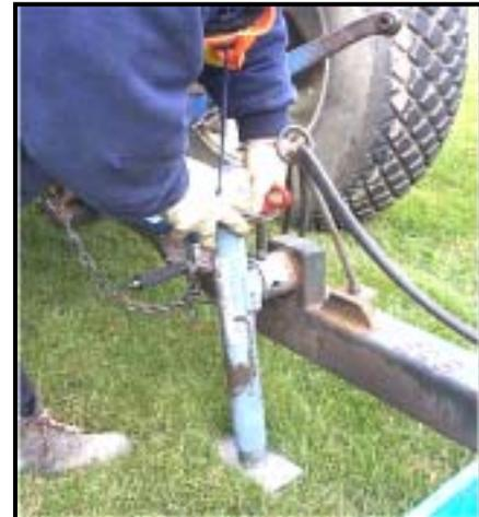
2. Next, insert the steel pin into the hole of the tractor and aerator hitches.
