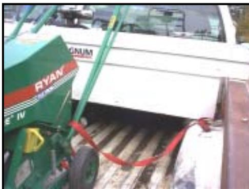
Just as you did when you unloaded the machine from the back of the truck, get a co-worker to help you lift the aerator into the back of the truck. Remember to bend your knees as you lift. Once the aerator is positioned in the truck, use four tie-down straps to secure the aerator to the truck ensuring it can't move around during transport.
