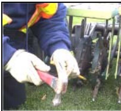
When the tubes/tines become clogged with soil, tap a piece of rebar into the tubes using a hammer. The soil will then be removed from the tube.
