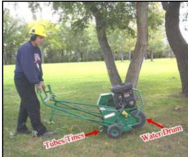
7. Before you make a turn, tip the aerator up onto the water drum, lifting the tubes/tines out of the ground.
